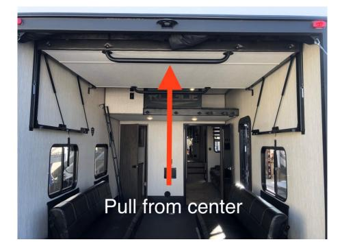
1. With the lock pins disengaged and starting on the vertical column side first, pull the bed down from the center most point until that side rests on the rubber bumpers.
