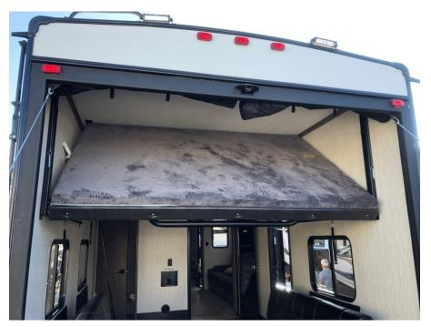
2. Go to the opposite side of the bed that is still up and pull down from the center most point of the bedframe until the whole bed is resting on the bumper rails. \*\*\*do not rest anything on bumper rail shelves and keep hands away from shelves while bed is being lowered!
